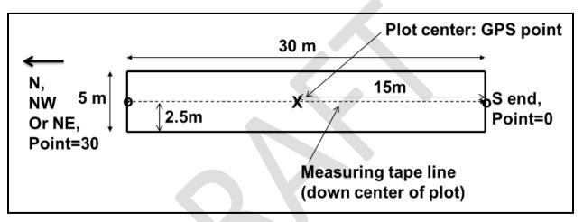
Figure 7.2. Diagram of a BEMP-style vegetation measurement plot proposed for vegetation monitoring.
