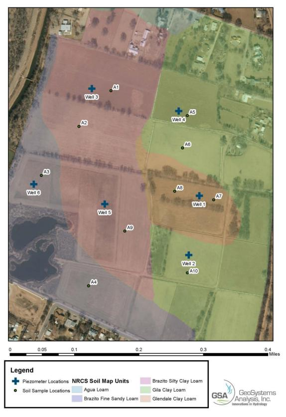
Figure 4.6. Soils map, including locations of soil samples and groundwater monitoring wells installed in 2018 (GeoSystems Analysis, Inc. 2018).
